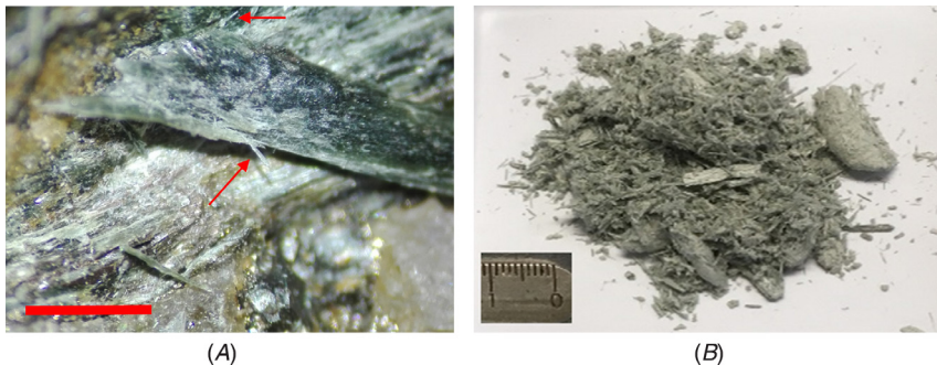
FIG. 4 (A) Two varieties of asbestiform amphibole, the first facies of amphibole varies in composition from ferro-actinolite to iron-rich actinolite. By scraping with a scalpel on the sides of these minerals, asbestiform fibers can come off (arrows); Bar = 0.5 mm. (B) Two varieties of asbestiform amphibole, the second amphibole facies is composed almost exclusively of acicular to asbestiform amphibole, the mineralogical composition of which varies from ferro-actinolite to magnesian actinolite.
