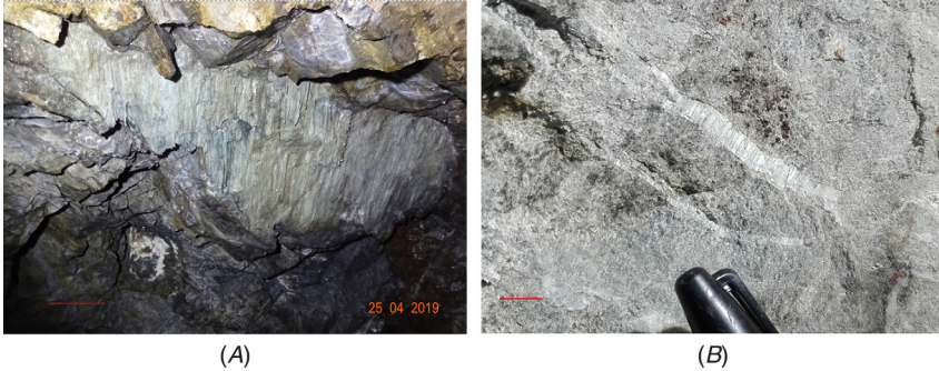
FIG. 3 (A) Dip-slip fault containing ferro-actinote “slip fibers” at level 1532, outside the exploration zone, the bar equals 15 cm, index 22 of company C1. (B) Crack-seal veins containing asbestiform actinolite cross fibers in the R1 drift of level 1230 of the exploration area.
